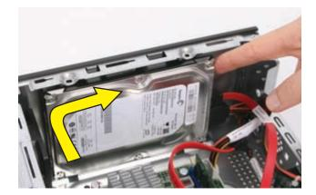
**6** Replace the hard drive retention screws and tighten them.
